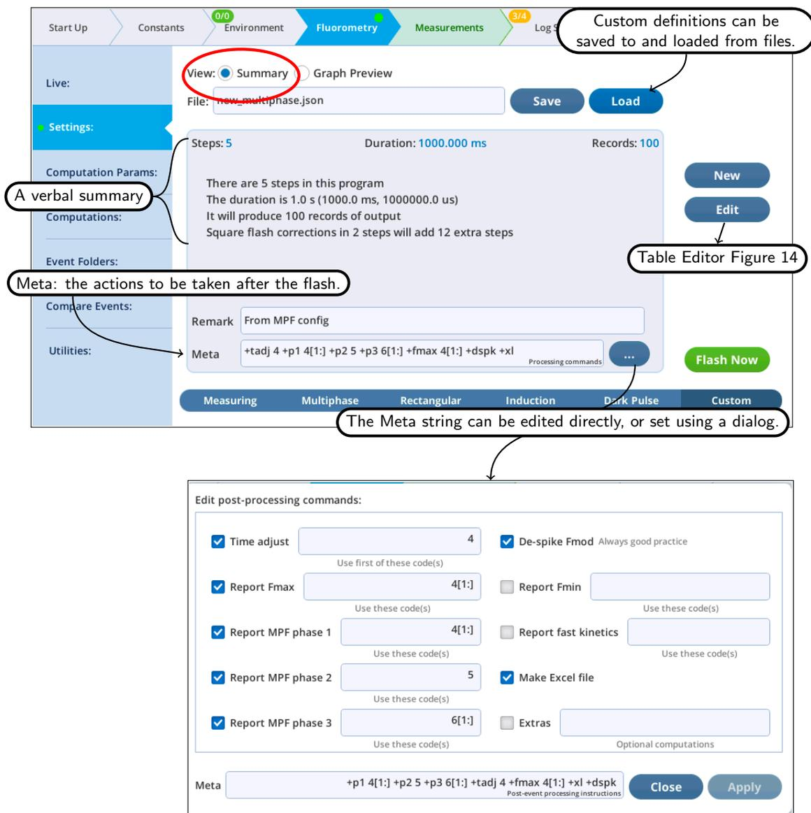
Figure 12: The Summary view provides a textual description, and the Meta string, which defines the post flash computations.
