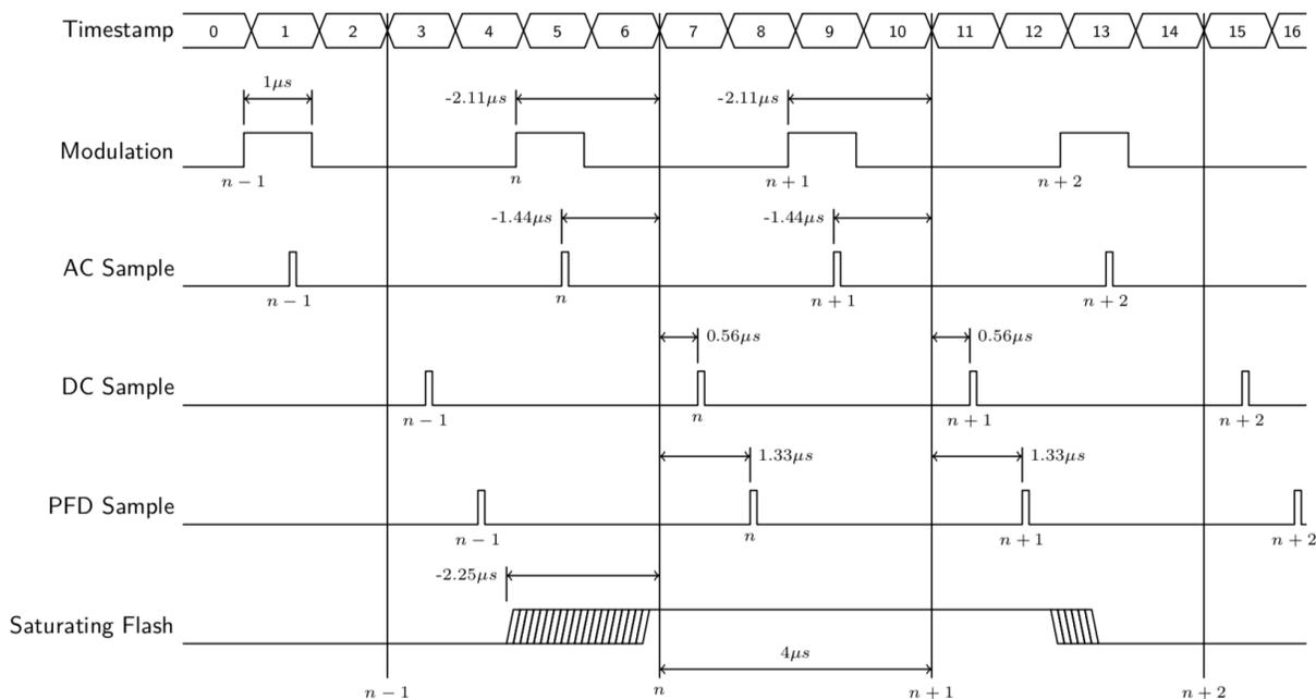
Figure 21: Timing when the modulating is set to 250000 Hz.
