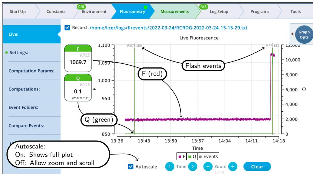
Figure 4: The **Live** screen shows a time-of-day strip chart of  $F$ ,  $Q$ , and fluorescence events.
