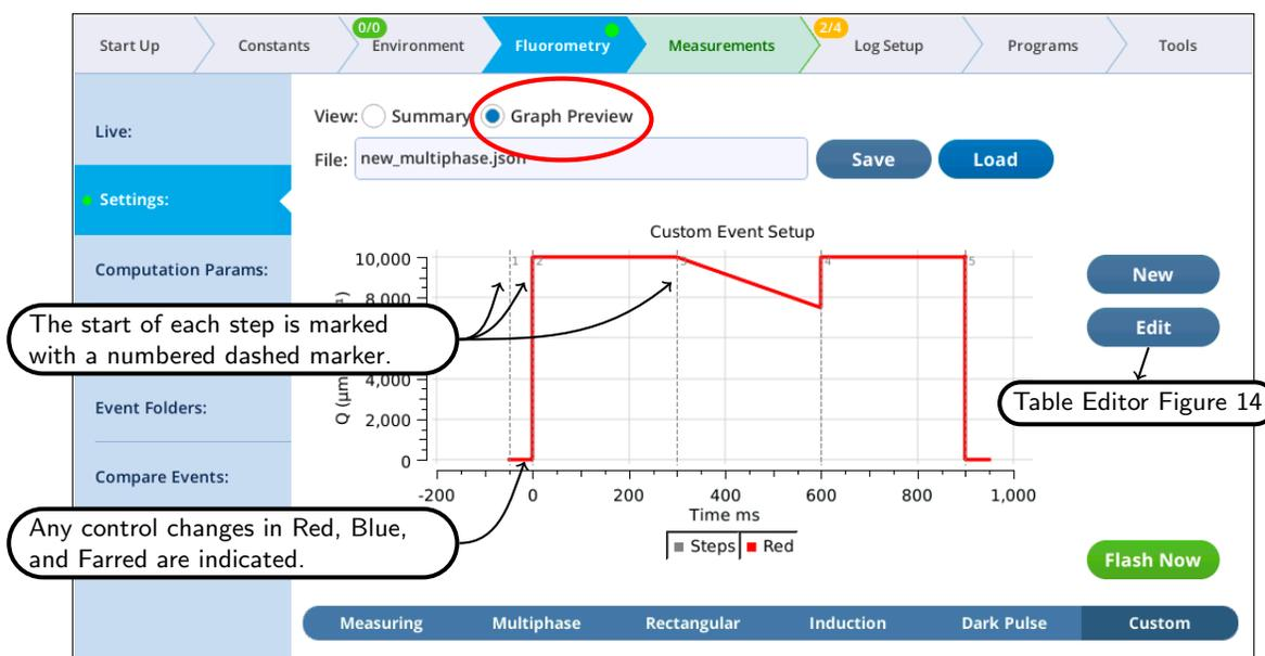
Figure 13: The Graphical view of a custom event shows the start time of each step, and any actinic light changes.
