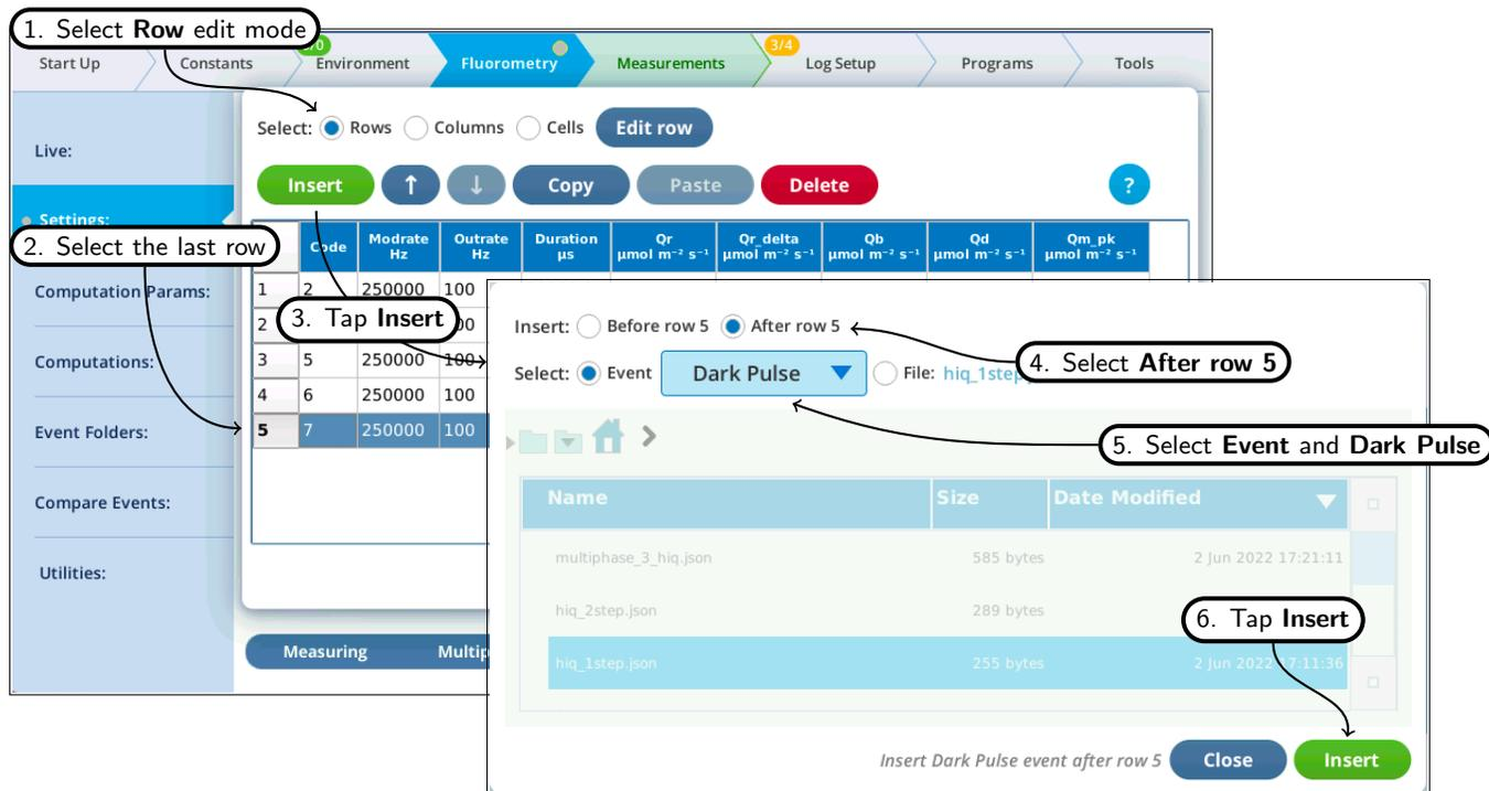
Figure 15: Step 3a. Appending a dark pulse to the custom flash step table.
