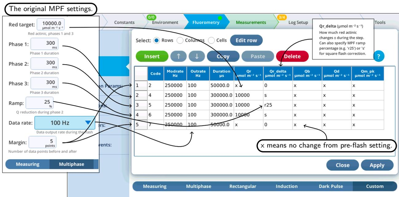
Figure 14: The Table Editor lets you view/edit what happens in the custom event at every step. For reference, we show the MPF settings that were used to generate the custom flash for this example.
