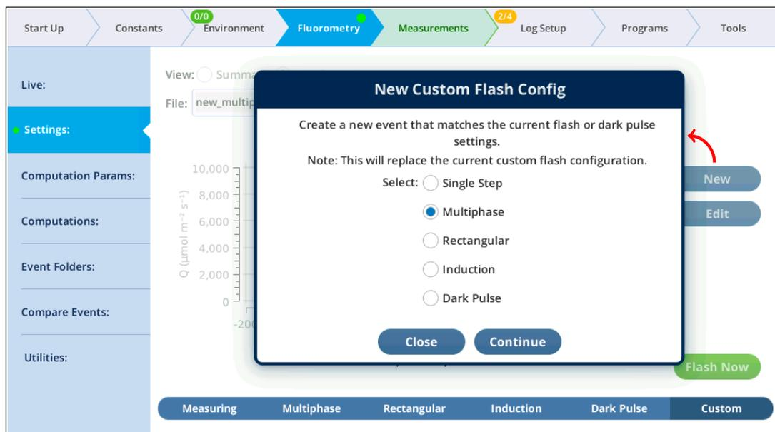
Figure 11: Make a new custom flash event that will match the current settings for the multiphase flash.
