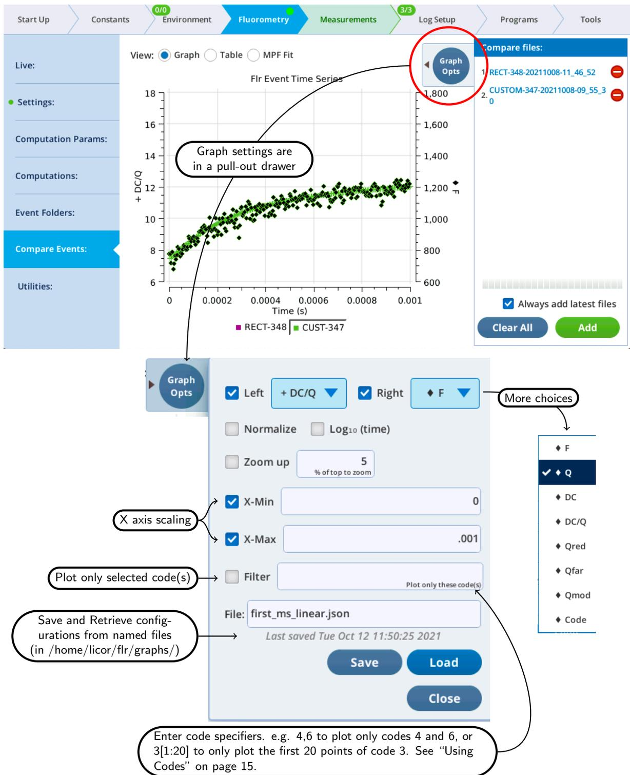
Figure 19: New graphing options for fluorometer event files.
